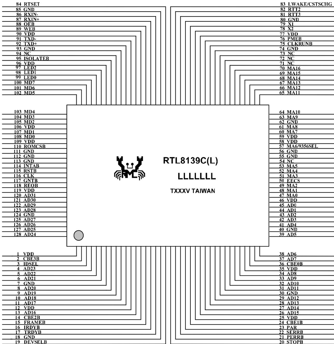
Figure 1. Pin Assignments
